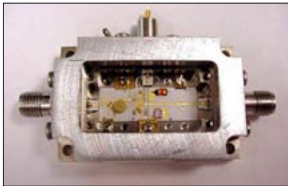
Fig. 1 A 12.5 GHz GaAs FET dielectric resonator oscillator (1.6" × 1" × 0.6"). ▼
